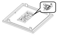
2. Plug the RJ11 connector of the LD-2100 cable into the LD-2100 I/O cable jack of the PP-7600X printer.
